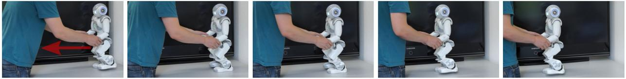
Fig. 6: The human directly guides the robot through longitudinal physical interaction. The robot infers the intended walking direction and adapts the walking parameters, i.e., heading and velocity, accordingly.
